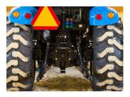
High Capacity Three Point Hitch Heavy-Duty Frame And Lift Cylinders Enable Three-Point Lift Capacity Of 2,755 lbs. At Hitch End
