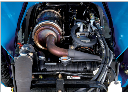
New LS Tier 4 CRDI Engine Meets EPA's most stringent emission standards while delivering rated horsepower quietly with low vibration
