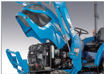
Easy open one-piece hood Provides accessibility for easy maintenance
