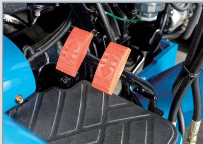
Hydrostatic transmission models Maximizes ease of use with effortless, clutch-less and instant speed and directional changes with a simple push of the pedal
