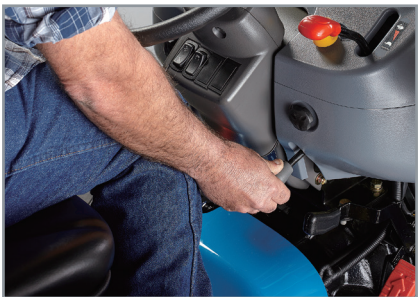
Tilt steering wheel Convenient lever allows you to adjust the tilt for maximum comfort
