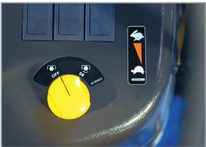
PTO On/Off switch Best easy and safety Independent PTO control with electric on/off switch. User friendly design and location for simple PTO operation.
