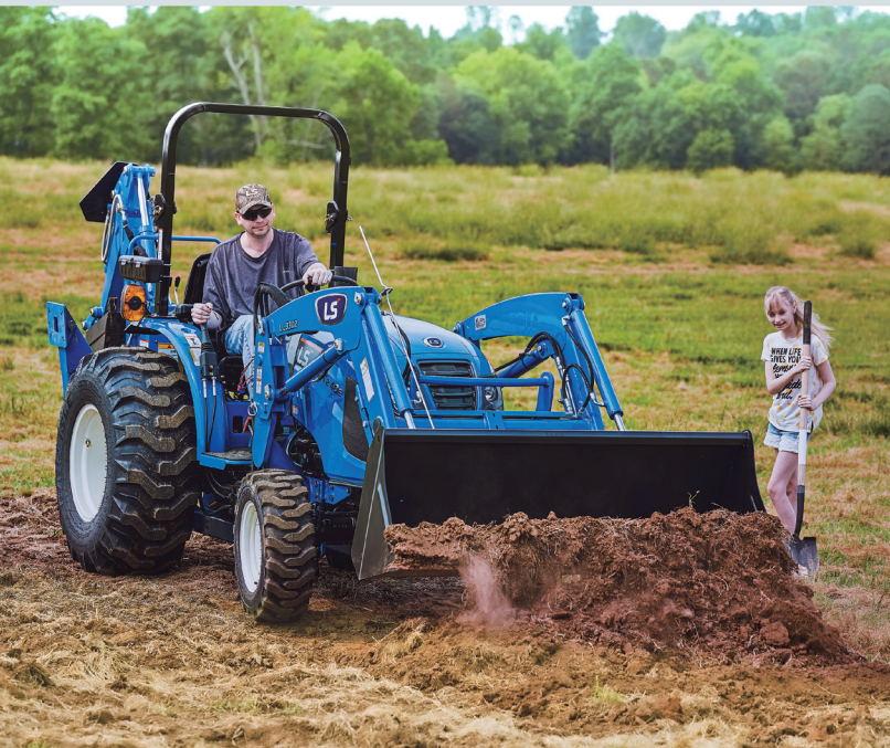
SKC bucket, front end loader with skid steer compatible bucket Easy to take off or attach loader and easily change loader attachments. With up to 2,153 lbs of lift capacity, it outperforms others in its class. Grill guard comes standard with loader rather than an option
