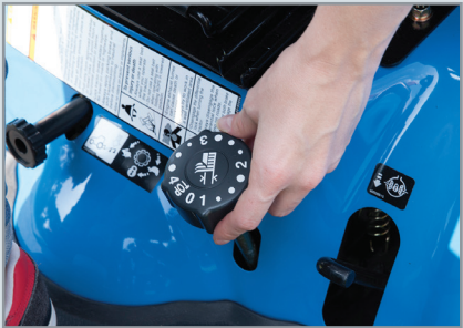
Easily adjust mowing height Adjusting the cutting height for the available 60" mid-mount mower is as easy as turning a dial.
