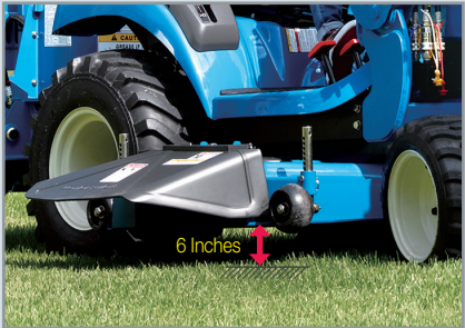
Excellent mower ground clearance The available mid-mount mower is easy to remove or attach and provide a full 6 inches of ground clearance
