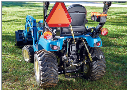
970 lb lift capacity The high lift capacity 3 point hitch is smooth and responsive
